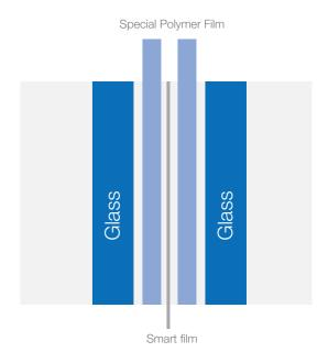
There is a smart film between the two Special Polymer films. The Smart Film is a suspension of liquid crystals in a polymer base that can be controlled using an electric charge. Under normal conditions the liquid crystals are randomly distributed and when light hits the glass, it is scattered by the liquid crystals.
