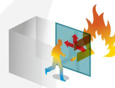
E 'Integrity' and ensures flames limitation': Restricts heat transfer to no more than 15 kW/m<sup>2</sup>
