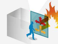
EI 'Integrity and Insulation': Blocks heat transfer
