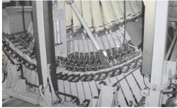
Picture 7. Example of the mouldless bending and tempering system for large glass sizes
