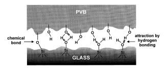
Figure 5. PVB-glass bonding mechanism.
