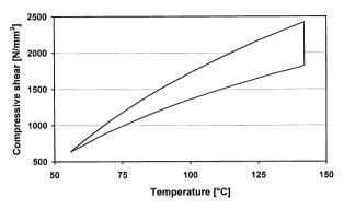
Figure 6. Compressive shear adhesion versus autoclave temperature.
