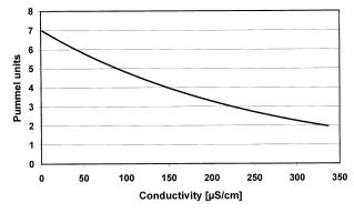
Figure 7. Pummel adhesion against conductivity of rinsing water.
