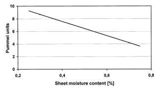
Figure 9. Pummel adhesion versus sheet moisture content.
