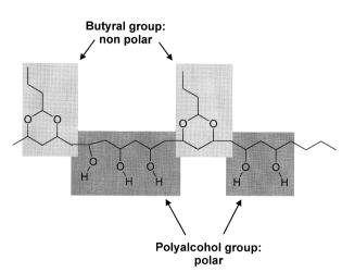
Figure 4. Chemical structure of PVB.
