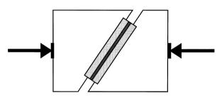
Figure 2. Position of the test specimen in the compressive shear test.
