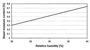
Figure 10. Sheet moisture content against relative humidity.
